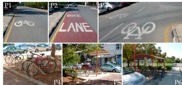
Figure 5. Quality of bike lanes and stations: P1-P2-P3 Insufficient and unsafe bike lanes only partially painted with no appropriate separation from motorized vehicles; P4-P5-P6 Bike stations and racks lacking of quality and safety within EMU Campus (Source: Authors).
