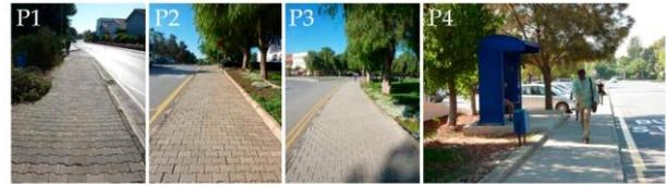
Figure 3. Quality of payments, shading elements and width of pedestrian paths: P1 Quality of payments along pedestrian paths within EMU Campus; P2-P3 Trees being the only elements providing shade for pedestrians along the sidewalks; P4—Insufficient width of pedestrian paths along the main axis (Source: Authors).
